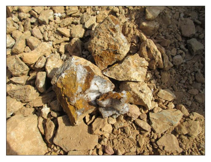
Figure 4: Rock chip sample of quartz veins from spoil pile which returned 79.50g/t Au
